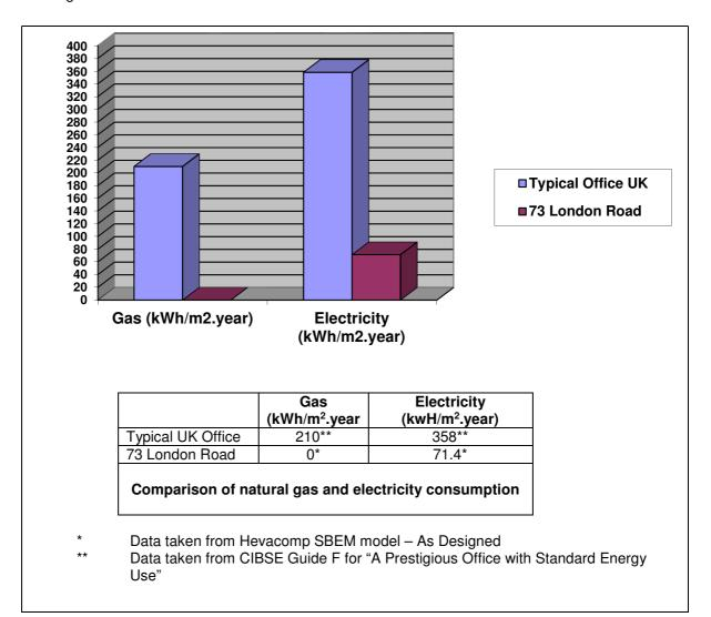
It is expected that consumption of natural gas will be 100% lower than a typical UK office building for 73 London Road, as all heating and domestic hot water will be produced by electric heat pumps.
